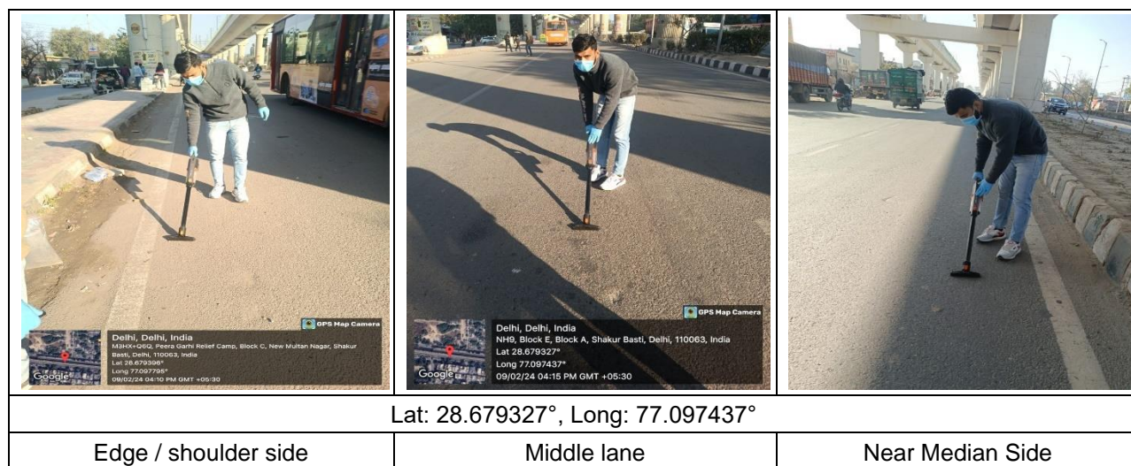
Plate 2.2: Photographs showing Road dust collection from Peeragarhi (NH-9) for particle size analysis
